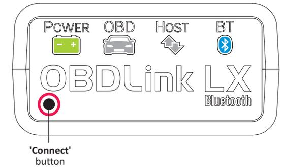
The 'BT' LED will switch to a *fast* blink.
