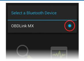
Once the app establishes a connection with MX, the 'BT' LED will turn on solid. Tap 'Diagnostics' to start a scan.
